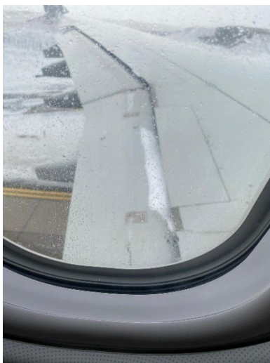
Figure 74 Example of contamination on hidden surface, post-de-ice
