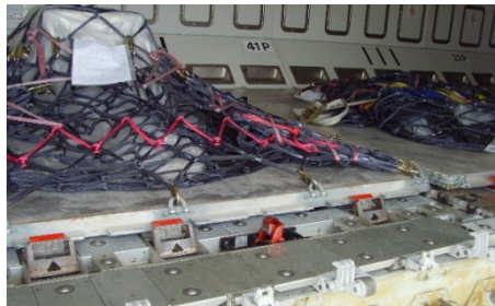
Figure 33 Example of military SL4 type ULD locked in position using the SL4 lateral locks
