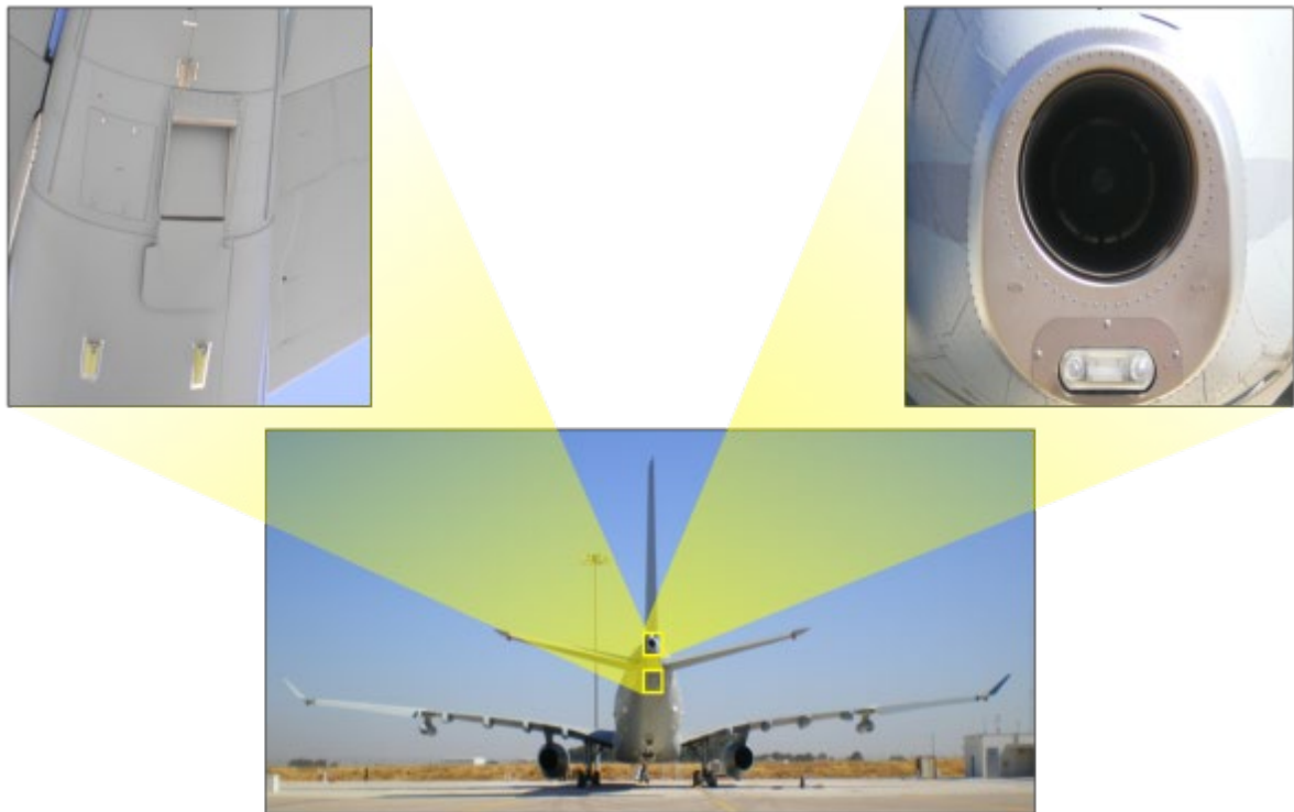
Figure 59 APU air intake and exhaust
