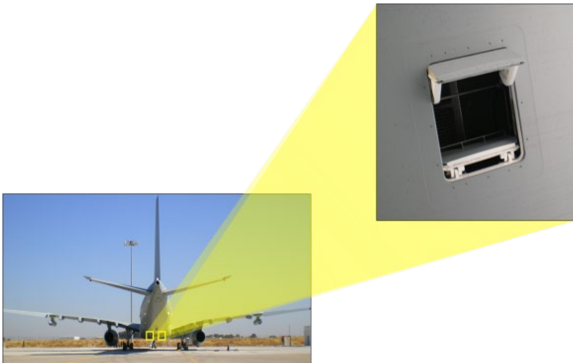
Figure 61 Outlets of fwd and aft outflow valve
