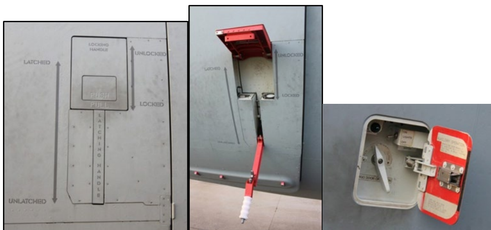
Figure 20 Operation of ULD Locks
