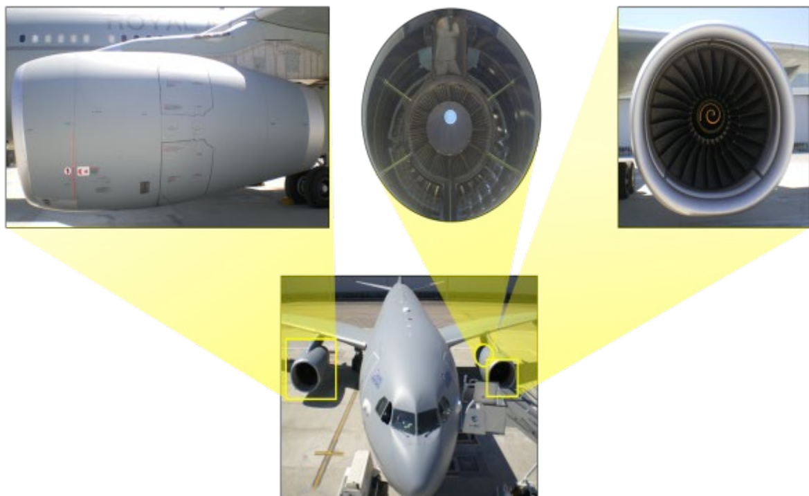
Figure 60 Engine cowls, air intakes and exhausts
