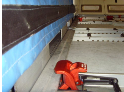
Figure 32 Example of AKE (LD3) type ULD locked using a longitudinal (forward/aft) lock
