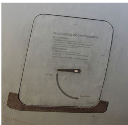
Figure 21 Bulk Hold Door Operation
