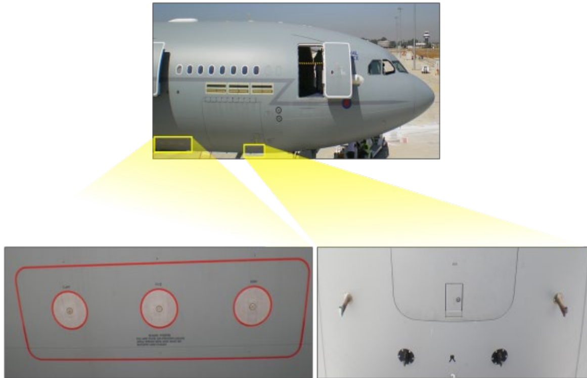
Figure 65 Static vents / probes
