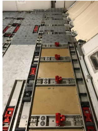
Figure 24 Example of a lateral, main compartment SL4 ULD lock
