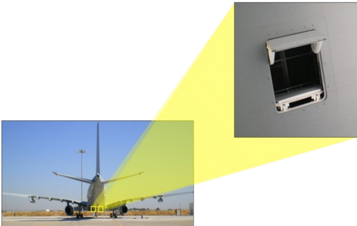
Figure 59 Outlets of fwd and aft outflow valve
