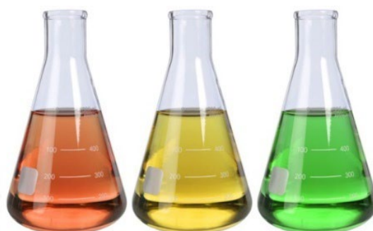
Figure 53 Fluid Types. The colours of the three most common types (I, II, and IV left to right, respectively) of aircraft de-icing/anti-icing fluids
