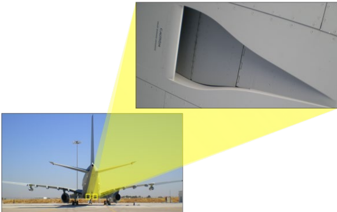
Figure 60 Outlets and inlets of the air conditioning system
