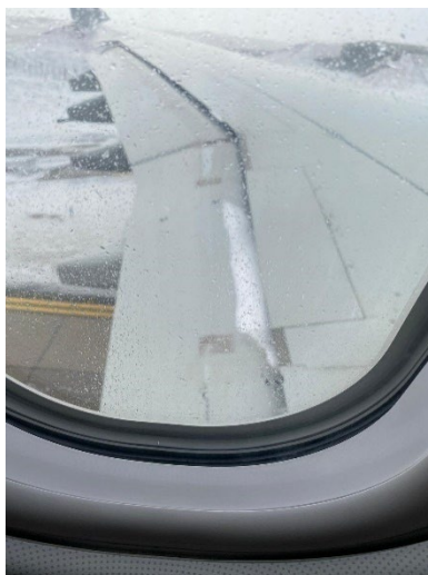
Figure 72 Example of contamination on hidden surface, post-de-ice
