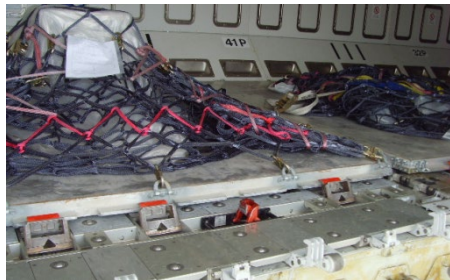
Figure 33 Example of military SL4 type ULD locked in position using the SL4 lateral locks
