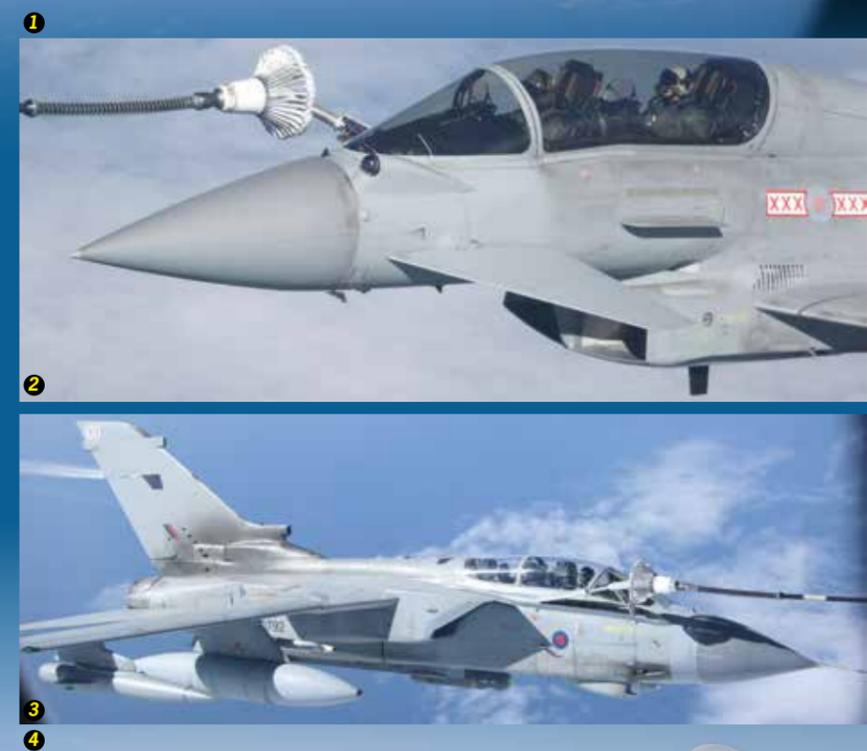
1: After heading northeast, 'Tartan 41' refuelled three 15(R) Sqn Tornado GR4s. 2: The back-seater of this 29(R) Sqn Typhoon T3 watches as the pilot plugs into the drogue just off the UK's east coast. 3: A Tornado GR4 takes on fuel from the Voyager, which can offload just over a ton of fuel a minute from the wing pods. 4: Having taken on fuel, this 29(R) Sqn pilot manoeuvres his Typhoon to the starboard wing and awaits the other jets in his formation. Photos, Alan Warnes
